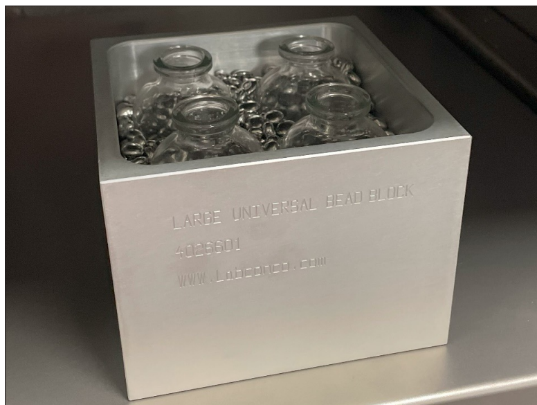
Figure 2: Labconco Large Universal Bead Block (4026601) and Lab Armor Beads for Universal Block (4026602) shown inside a FreeZone Triad Freeze Dryer (794001010).
